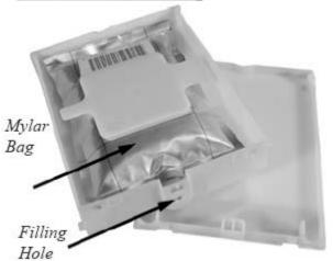
Fill the syringe with the correct color ink and carefully insert the needle into the filling hole / access port and slowly inject approximately 90 ml of ink into the cartridge. Unused ink may be returned to the bottle.
